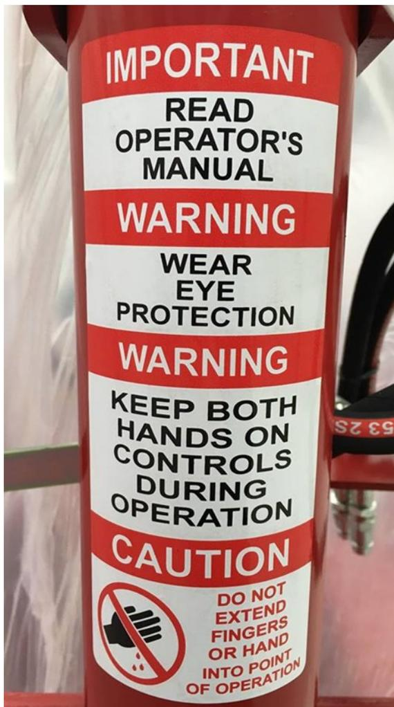
This safety decal is on the hydraulic ram and should be replaced if missing or becomes illegible.
